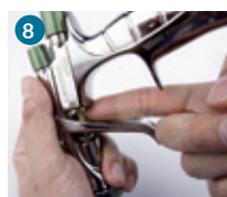
8 Grease the air valve bar behind the trigger
