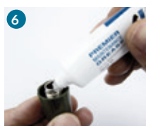
6 Grease the threads of fluid adjustment knob
