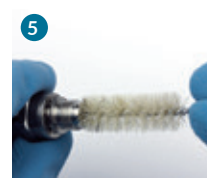
5 Clean smoothly the internal nozzle part, by using the most suitable brush size
