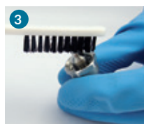
3 Clean the tip of the fluid nozzle carefully with a brush
