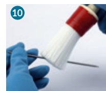
10 Clean the fluid needle with the most suitable brush
