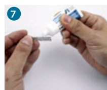
7 Grease the needle spring sections and insert it in its seat
