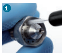
1 Clean the fluid nozzle small holes with a tiny twisted brush ø 3 mm
