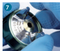
7 Clean the tiny air cap holes with the most suitable cleaning needles size
