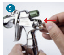
5 Insert the fluid needle in its seat
