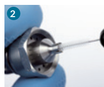
2 Clean the central nozzle orifice with a tiny twisted brush ø 3 mm
